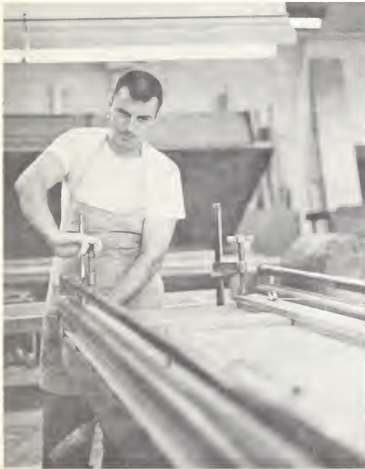
Figure 2.--Considerable skill is required of this employee at the Baxter Company in Duluth. He is placing a plastic overlay on particleboard to be used in a counter top. Skilled occupations accounted for nearly one-fourth of those employed in the study counties in 1960.
